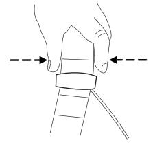
2. If you plan to carry very large objects or items that might damage the center lap/shoulder belt, detach the belt from the seat. Use a key or seat belt tongue to release the buckle.
